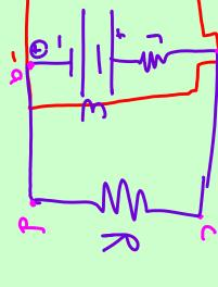
The load resistance is the resistance of the external resistor.
